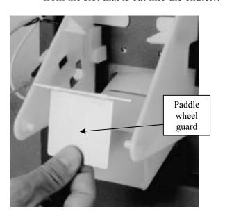
11 ...and remove the paddle wheel guard retainer.
